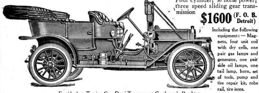
Four cylinder; 30 horse power; three speed sliding gear transmission
