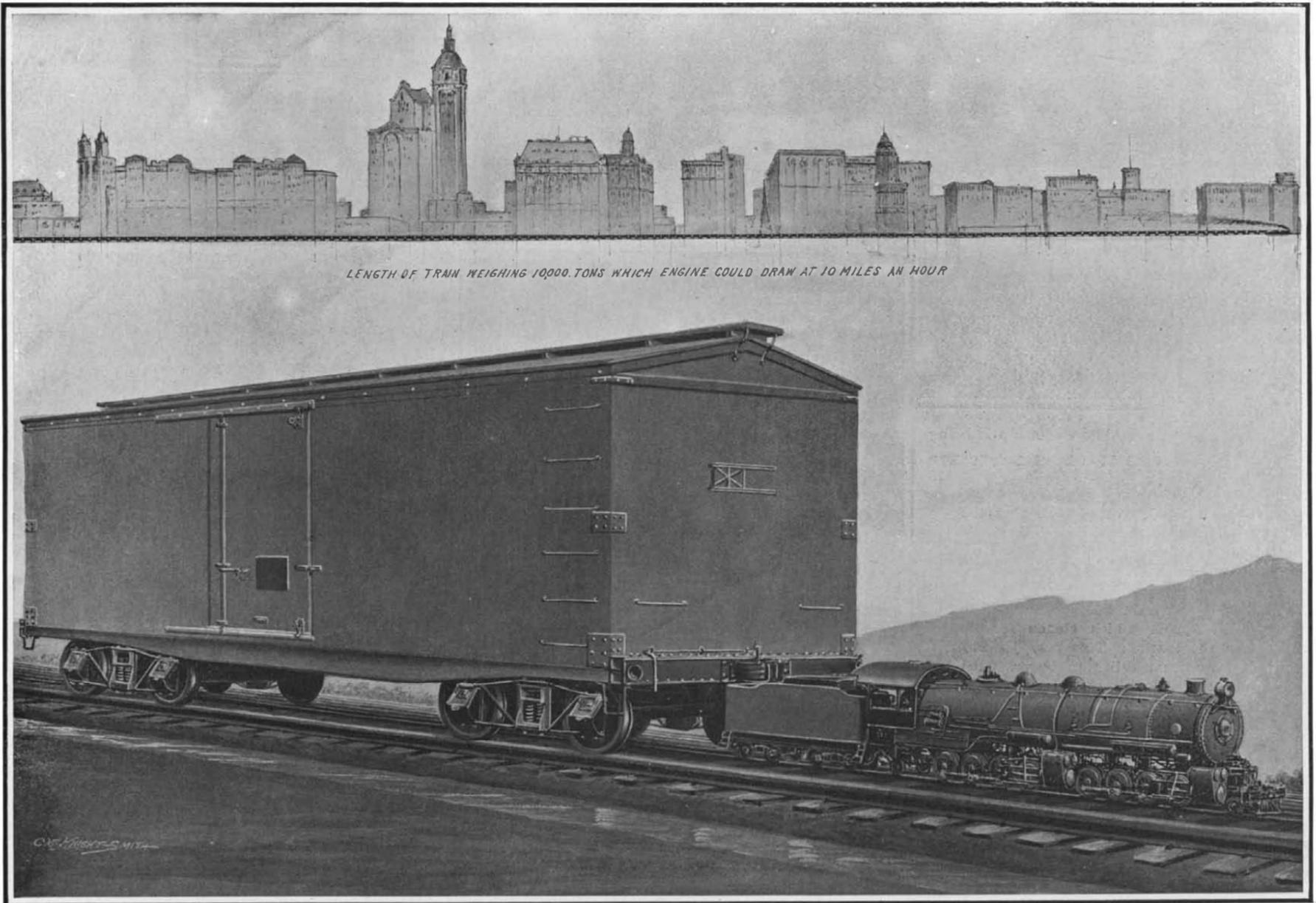
This huge Baldwin freight engine, weighing 300 tons, was built for the Southern Pacific Railroad. It is capable of hauling at 10 miles an hour a train of 169 cars weighing, with load, 72 tons each. The train, weighing 10,000 tons, would reach for over a mile or, say, from City Hall Square to the Battery, New York. The lower cut represents the size of a single car, 200 feet by 45½ feet by 62 feet, that would be necessary to contain the load of wheat handled.
