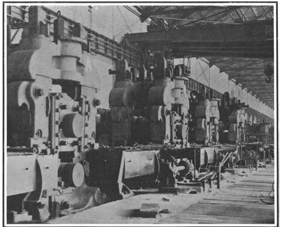
Contains four 40-inch blooming mill stands each driven by a 2,000-horse-power electric motor and a 32-inch mill driven by a 6,000-horse-power motor.
