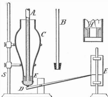
**APPARATUS FOR ILLUSTRATING THE "HYDROSTATIC PARADOX."**
