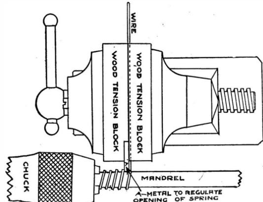
METHOD OF WINDING AN OPEN SPRING.
