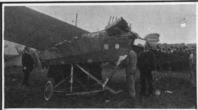
Front view of Latham's monoplane, showing damage sustained in alighting.
