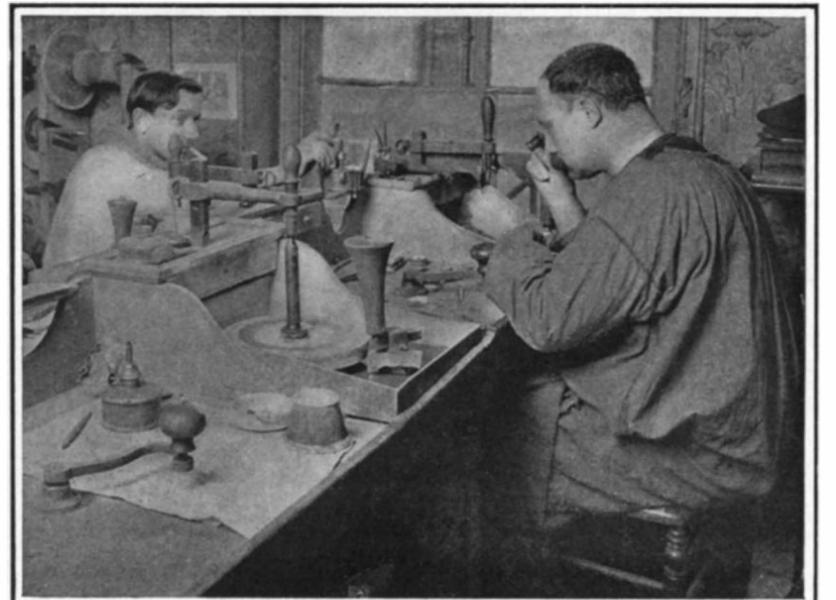
Fig. 4.—Examining artificial rubies, and mounting them on rods for cutting.
