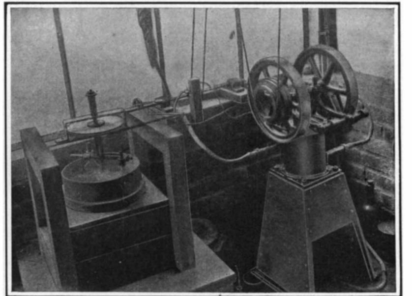
Fig. 1.—Sifting the mixture of alumina and oxide of chromium.
