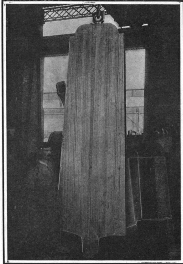
An 18-ton ingot sawn in two to show absence of piping.
