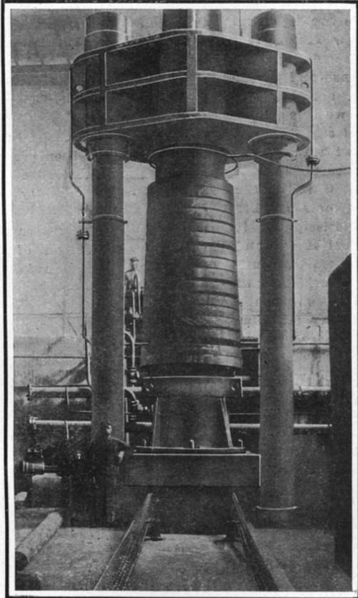
A 3,500-ton fluid-compression press capable of taking a 22-ton ingot.
