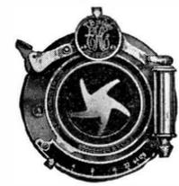
A feature of the 1909 model is the Kodak Ball Bearing Shutter, in which we have embodied a new principle in shutter construction. The leaves are in five segments, mounted entirely on ball bearings and open in the form of a star, thus admitting a much greater amount of light in a given time than any other between the lens type of shutter. Practically frictionless and with a precision and smoothness that are a mechanical delight.
