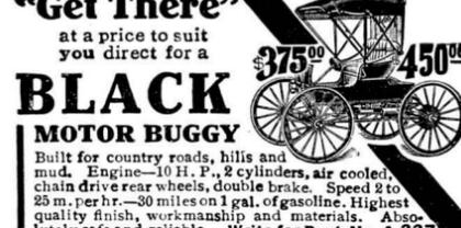
Built for country roads, hills and mud. Engine—10 H. P., 2 cylinders, air cooled, chain drive rear wheels, double brake. Speed 2 to 25 m. per hr.—30 miles on 1 gal. of gasoline. Highest quality finish, workmanship and materials. Absolutely safe and reliable. Write for Book No. A-227
