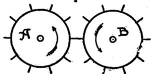
distances around the rim, as shown in above sketch. Now if one disk is made to revolve 10,000 R. P. M., while the other is stationary and in a position where one of its blades would come in contact with each of the revolving blades, there would be 100,000 contacts made per minute. Now if both disks were revolved in opposite directions, at exactly the same speed, 10,000 R. P. M., would the number of contacts remain the same, or
