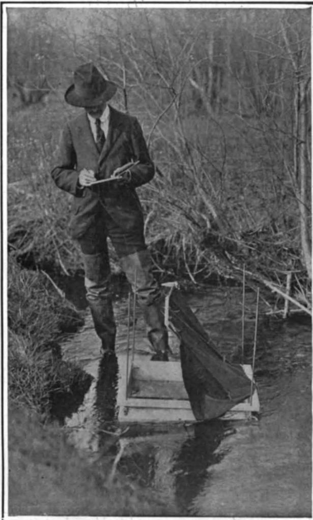
Fig. 3.—Two-foot water glass for studying lampreys.
