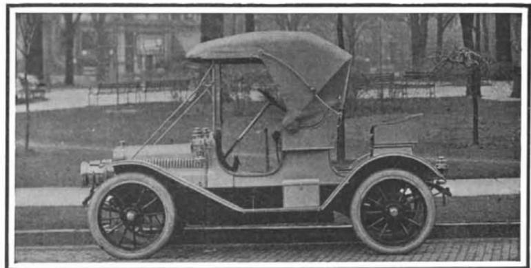
Wheel base, 95 inches; 18-20 horse-power motor; thermo-syphon cooling; mechanical oiler; jump spark ignition; friction transmission; pressed steel frame.
