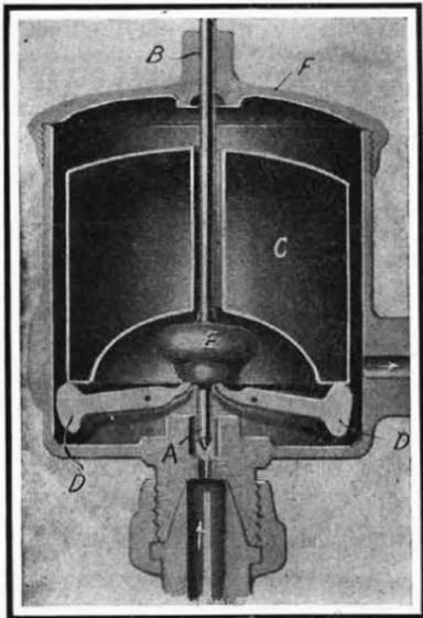
**CORRECTING A LEAKY CARBURETER FLOAT VALVE.**
