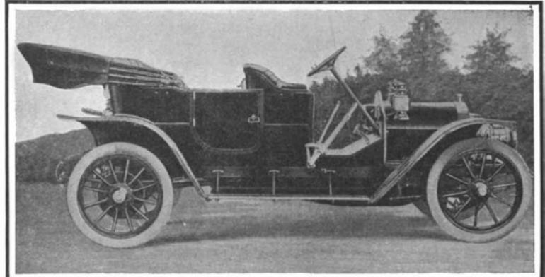
4 cylinders cast integrally; short bonnet; long wheel base; body swung between axles to give ease in riding; ignition by storage battery and coil; special equipment for double ignition (magneto with separate set of spark plugs).
