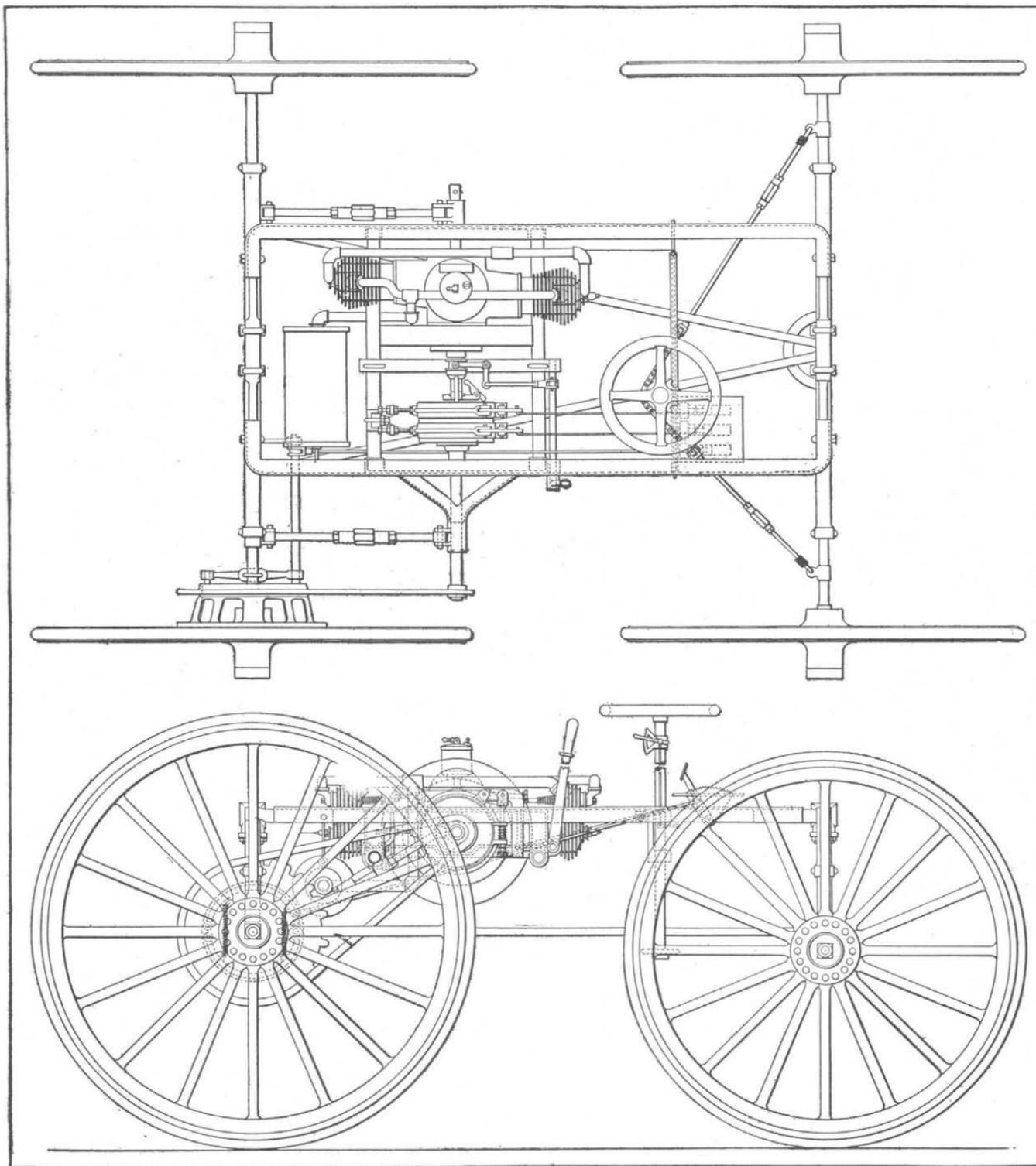
PLAN AND SIDE ELEVATION OF THE ASSEMBLED BUGGY.
