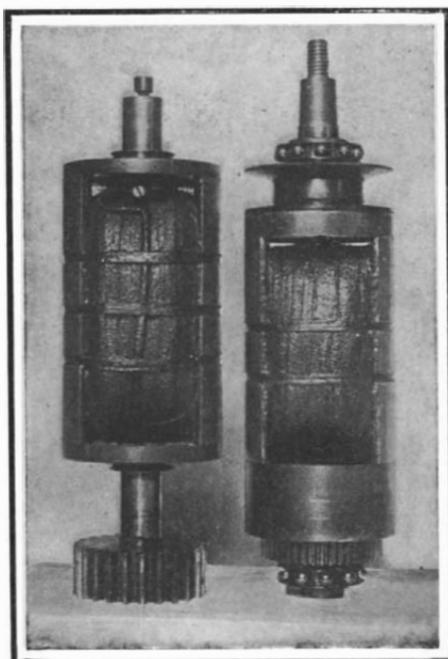
Fig. 5.—Typical magneto armatures.
