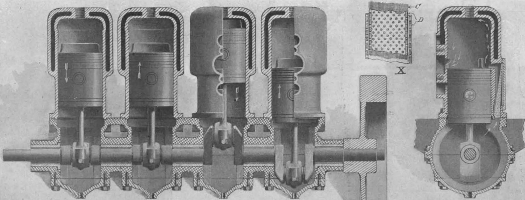
Fig. 4. TWO-CYCLE, THREE-PORT - ELMORE MOTOR
