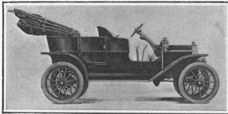
Wheel base, 100 inches; 4 cylinders; spur planetary transmission; low tension magneto ignition; vanadium steel springs, axles, shaft, gear, etc.; weight, 1,200 pounds.
