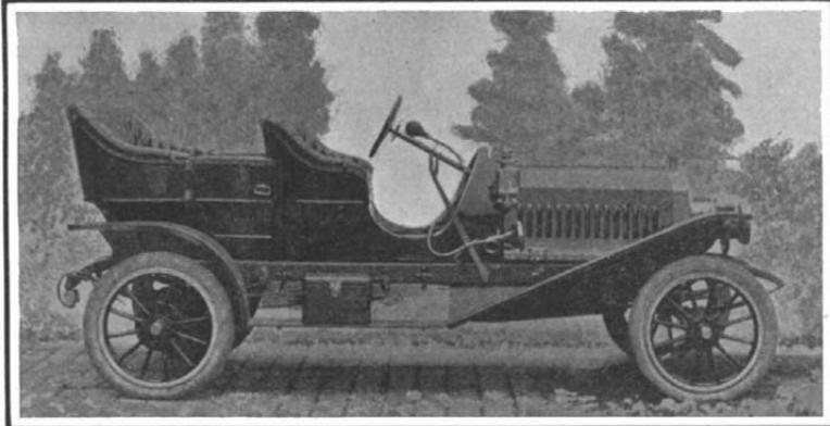
Wheel base, 110 1/4 inches; 28 horse-power; 4 cylinders, 4 x 4 inches; water cooled; jump spark ignition (storage battery); splash lubrication; single silent chain drive inclosed in dust-tight metal case; friction change gear.
