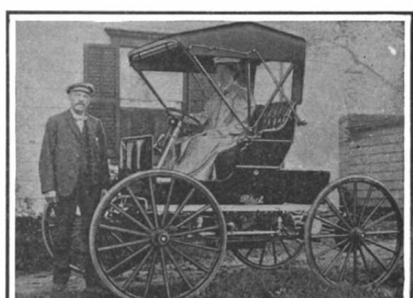
2-cylinder, 14-horse-power engine; planetary transmission; two speed forward and one reverse; maximum speed, 30 miles.
