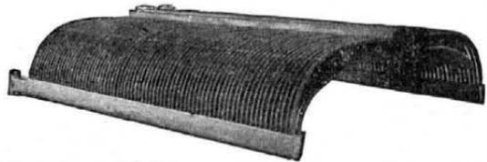
This Radiator is 12' 6" long by 4' 3" between centers. Contains 2,138 square feet of radiating surface. Constructed of 3/8" No. 18 Rome Seamless Copper Spiral Tubing.
