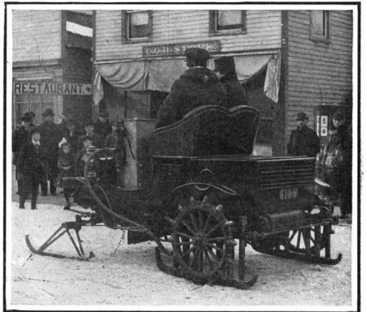
An attachment by means of which any automobile can be converted into a sled.
