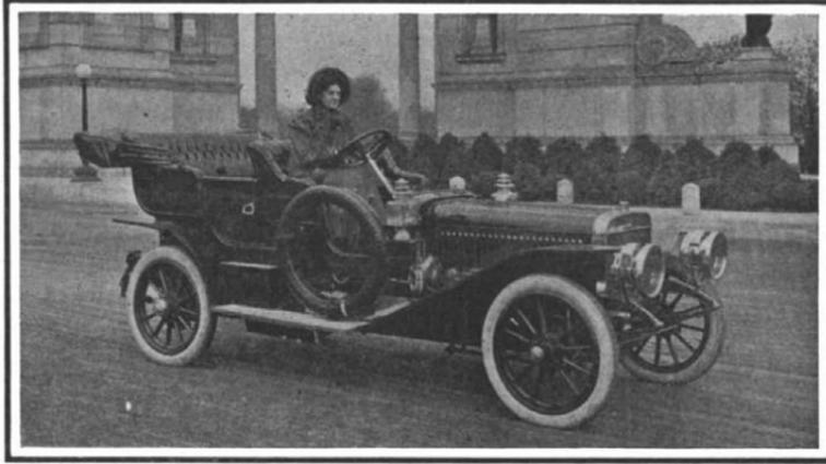
48 horse-power; 6 cylinders, vertical tube radiator; dry battery and high-tension magneto ignition; multiple-disk clutch; selective sliding gear transmission; shaft drive.
