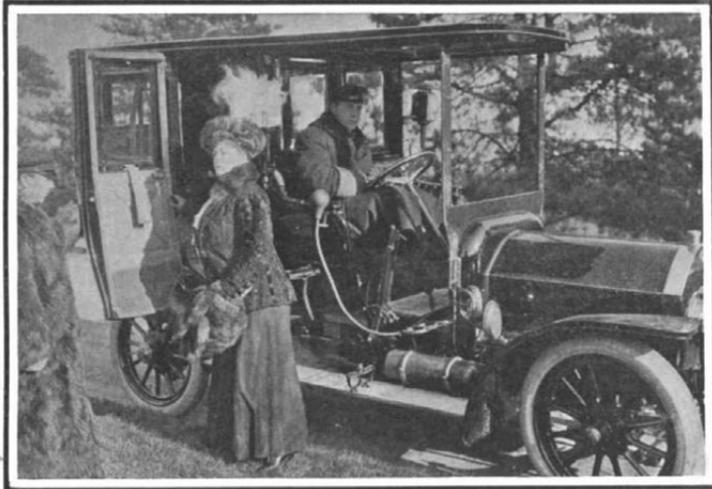
Wheel base, 117 inches; 40 horse-power; 4 cylinders, 4 3/4 x 5 1/4 inches; cellular radiator; low-tension magneto; cone clutch; selective sliding gear transmission with four speeds forward and one reverse; shaft drive.
