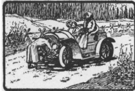
**Engine will not start.** { Test ignition and carbureter. { Slow cranking or cold weather will interfere with the proper formation of the mixture. { Prime cylinders with gasoline in cold weather to obtain mixture for starting. { To increase suction in carbureter, prevent operation of air-valve.
