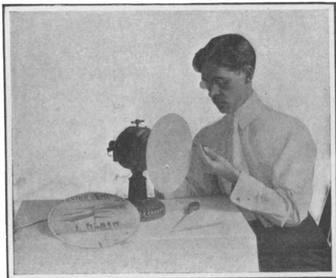
CUTTING A PENCIL WITH A DISK OF BRISTOL BOARD.
