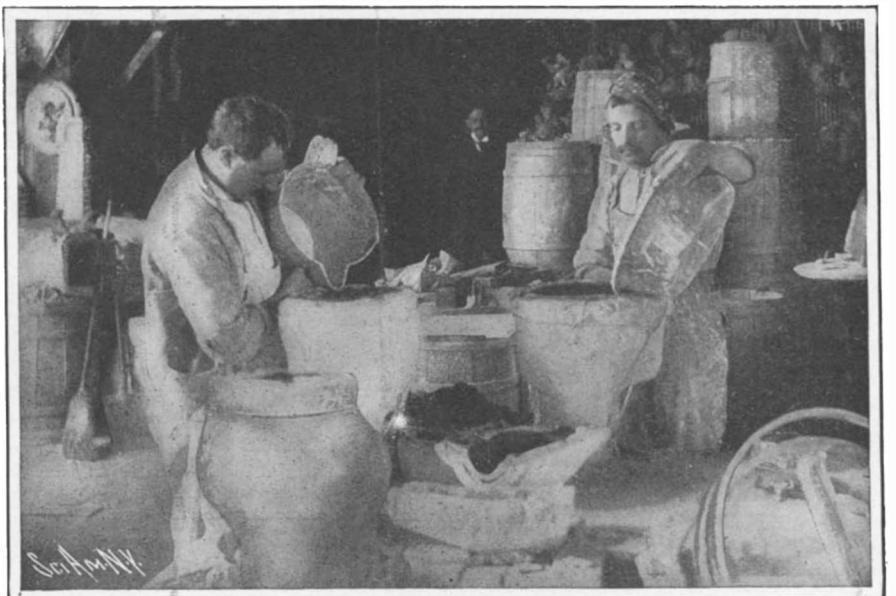
Pouring the Composition Into the Molds.
