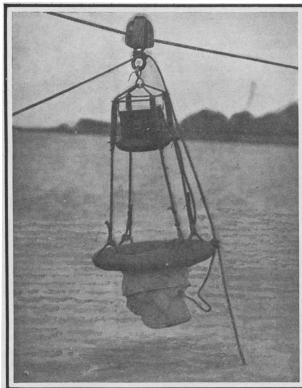
The Small Rubber Cushion Supports a Battery and Signal Lamps.
