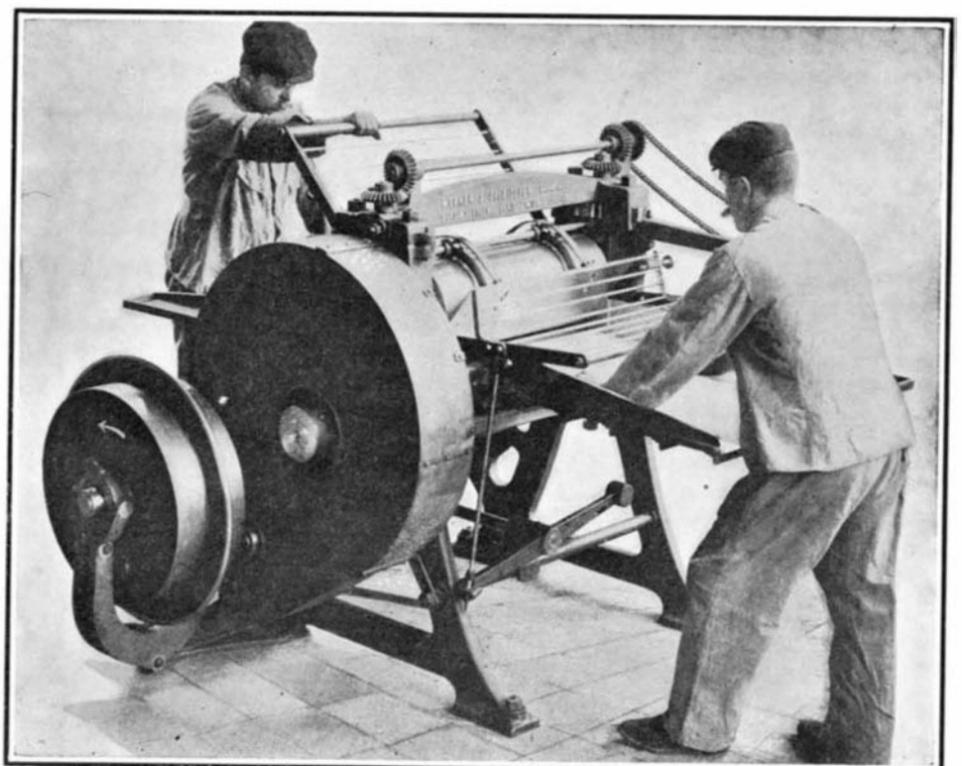
**A Dough-Working Machine Provided with Device to Prevent the Fingers of the Operator from Being Crushed Between the Rolls.**
