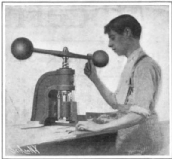
THE OLD METHOD OF PRINTING AND EMBOSSEING FROM STEEL DIES, IN USE FOR THE PAST CENTURY.
