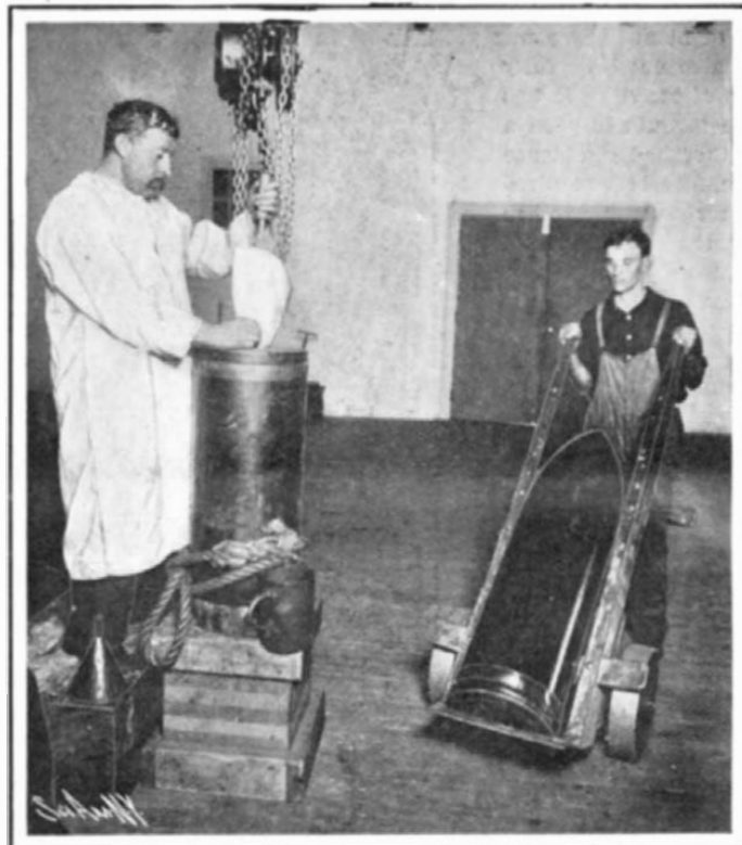
Putting in the Bag to Hold the Bursting Charge of 50 Pounds of Black Powder for a 13-Inch Shell.
