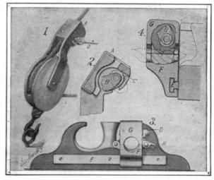
CHECK ATTACHMENT FOR PULLEYS AND CHOCKS.
