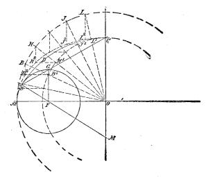
July 14, I beg leave to say that the figure submitted is not an ellipse at all, but merely a curve composed of the arcs of two pairs of circles.
