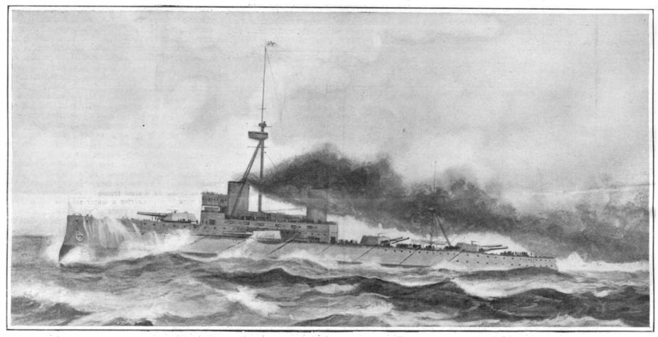
Length, 520 feet. Beam, 82 feet. Draft, 261/2 feet. Displacement, 18,000 tons. Speed, 21 knots. Armor: belt, 11 inches; turrets, 11 inches. Guns: ten 12-inch, eighteen 3-inch.
