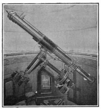
Double Equatorial Telescope.
