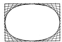
lipse can be made by the instrument called the ellipsograph, and by the "string," also by the following process: Square the length and width you desire your ellipse to be. Divide the sides and ends in thirteen equal parts, and draw lines as in the figure. By this process a perfect ellipse may be obtained of any size and shape.
