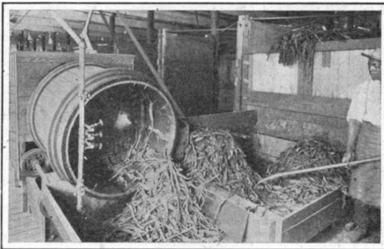
Fig. 3.—Spraying and Blending the Tobacco in the Mixing Cylinder.
