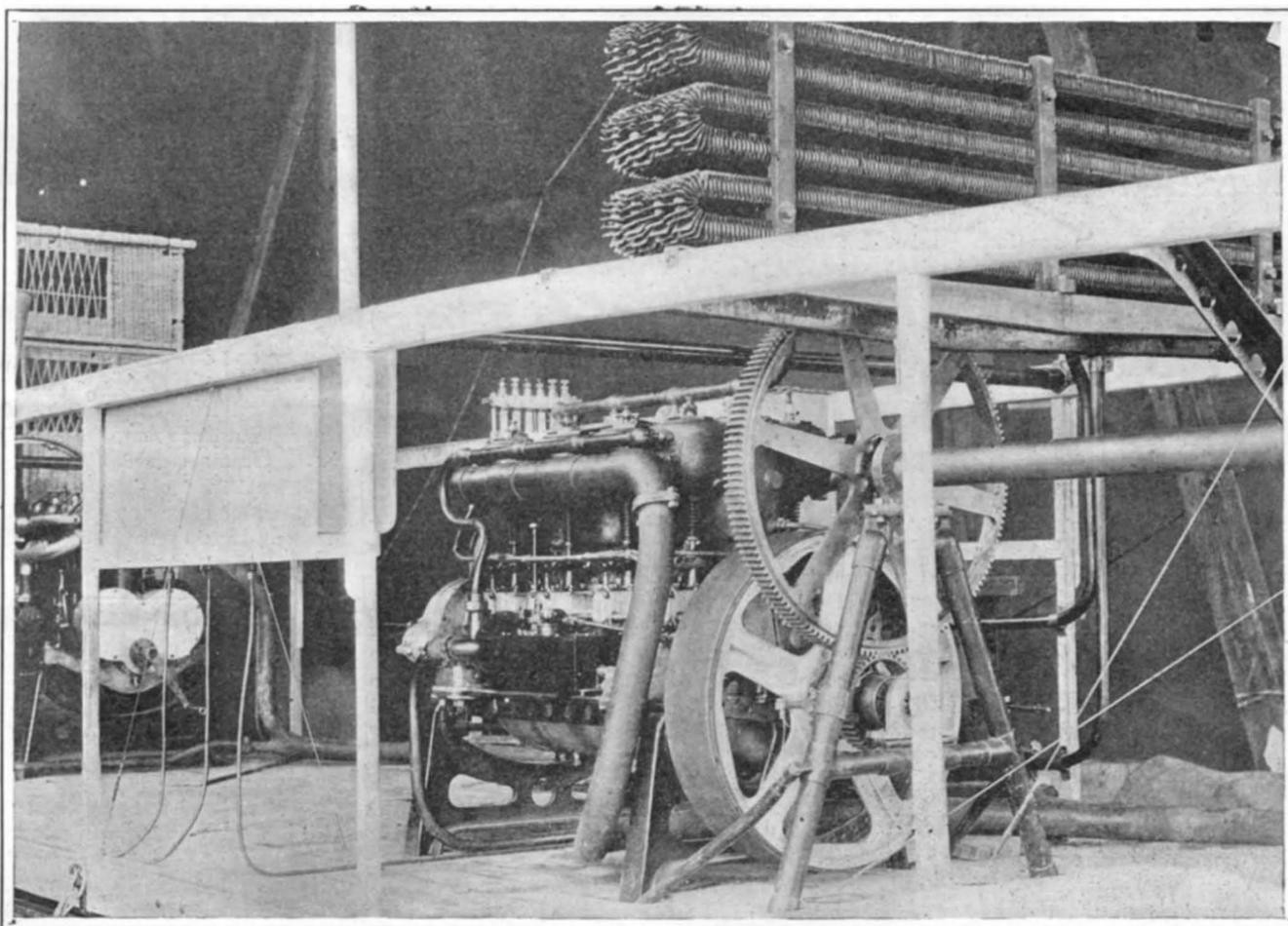
Center of Body, Showing Cabin on the Left, the Two Motors and Radiator, and the Gears Which Drive the Forward Propeller Shaft.
