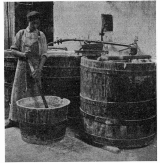
Fig. 2.—Mixing Colors with Stearine.
