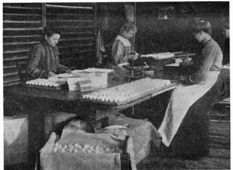
Fig. 7.—Cupping, Labeling and Packing Night Lights.
