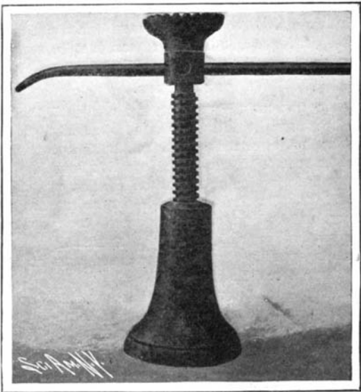
Jack-Screw Used to Lift Safes Into the Proper Position to Blow Them Apart.
