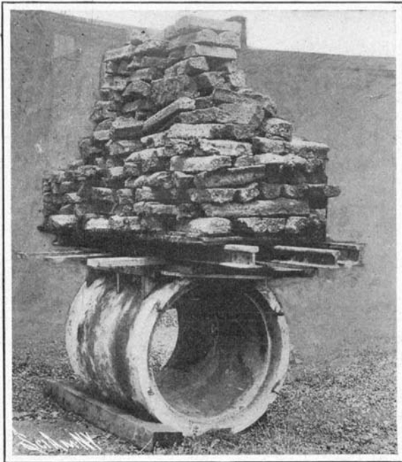
Section of 36-Inch Reinforced Concrete Pipe, 90 Days Old, Carrying Weight of 20,000 Pounds.
