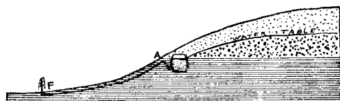
Fig. 4.—METHOD OF CONSTRUCTION OF "GEYSER SPRINGS."
