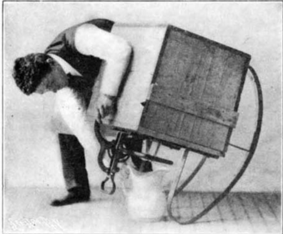
TILTING A CARBOY EQUIPPED WITH AN INCLINATOR.
