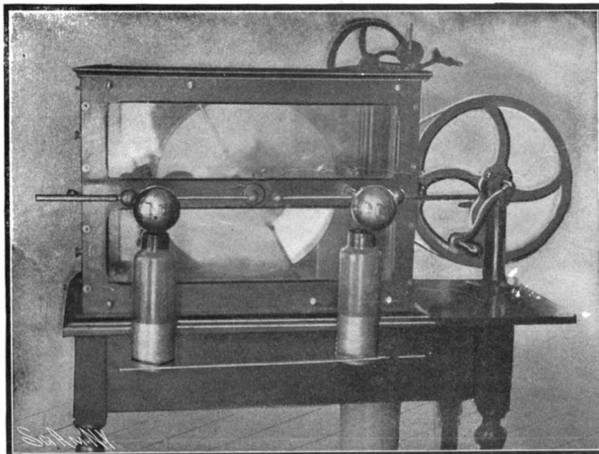
STATIC ELECTRIC MACHINE USED IN EXPERIMENTALLY DISPELLING FOG BY ELECTRICITY.
