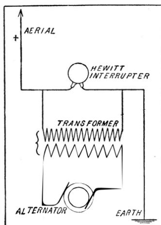
Electrical Connections of the Fog Dispersing Apparatus.
