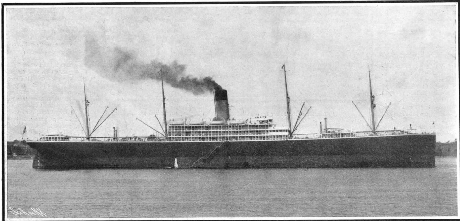
Length, 630 feet. Beam, 73 feet. Displacement, 37,000 tons on a draft of 36½ feet. Speed, 15 knots.
