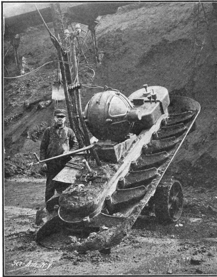
3. Screw for raising and lowering front of machine. 4. Steering lever.
