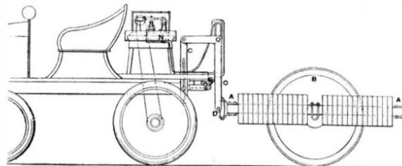
THE DYNAMOMETER APPLIED.
