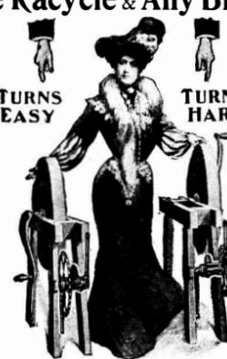
Racycle sprockets turn between bearings. Bicycle sprockets turn outside bearings.
