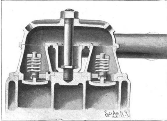
**METHOD OF SECURING INLET VALVES.**
