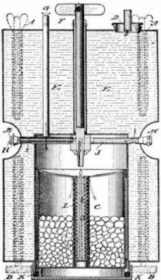
CROSS-SECTION OF ACETYLENE LAMP.
