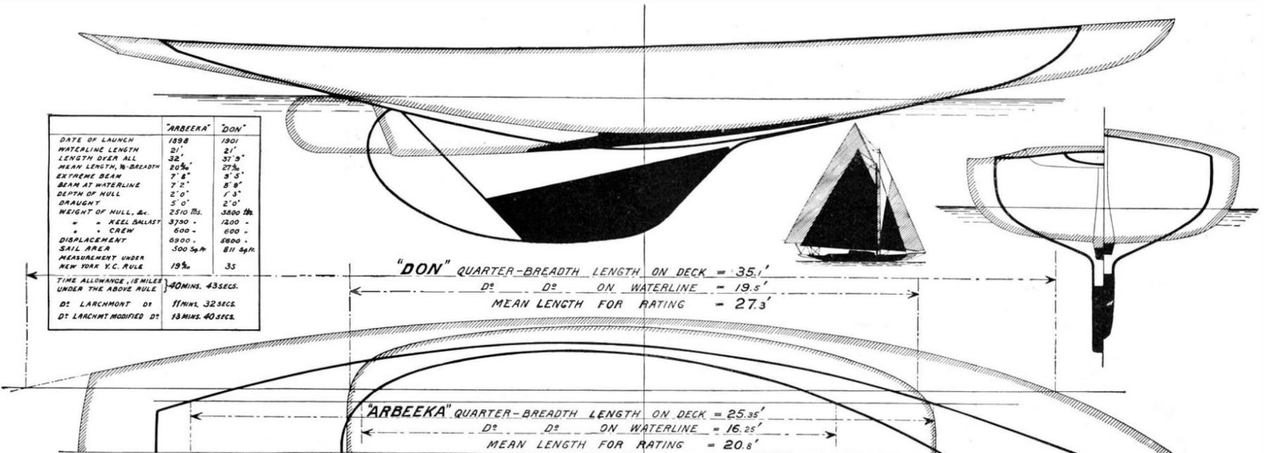
DIAGRAM SHOWING THE EXTENT TO WHICH THE N. Y. Y. C. NEW RULE OF MEASUREMENT TAXES THE EXAGGERATED PROPORTIONS OF A MODERN SCOW-TYPE RACING CRAFT.
