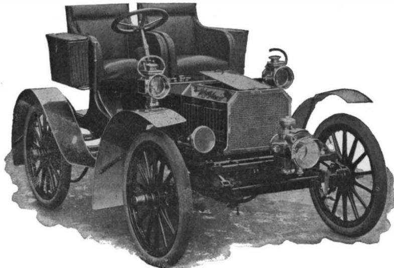
Wheel Base, 6 ft.6 in.; Wood Wheels; Cone Clutch; Sliding Gear. Transmission, 3 Speeds Forward and Reverse, 1st, 12 miles; 2d, 20 miles; 3d, 35 miles.
