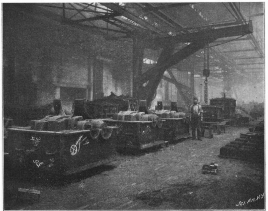
**The Foundry, Showing Flasks for Compound Cylinders.**
