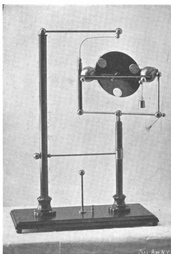
Fig. 2.—BOHNENBERGER APPARATUS DRIVEN BY STATIC ELECTRICITY.
