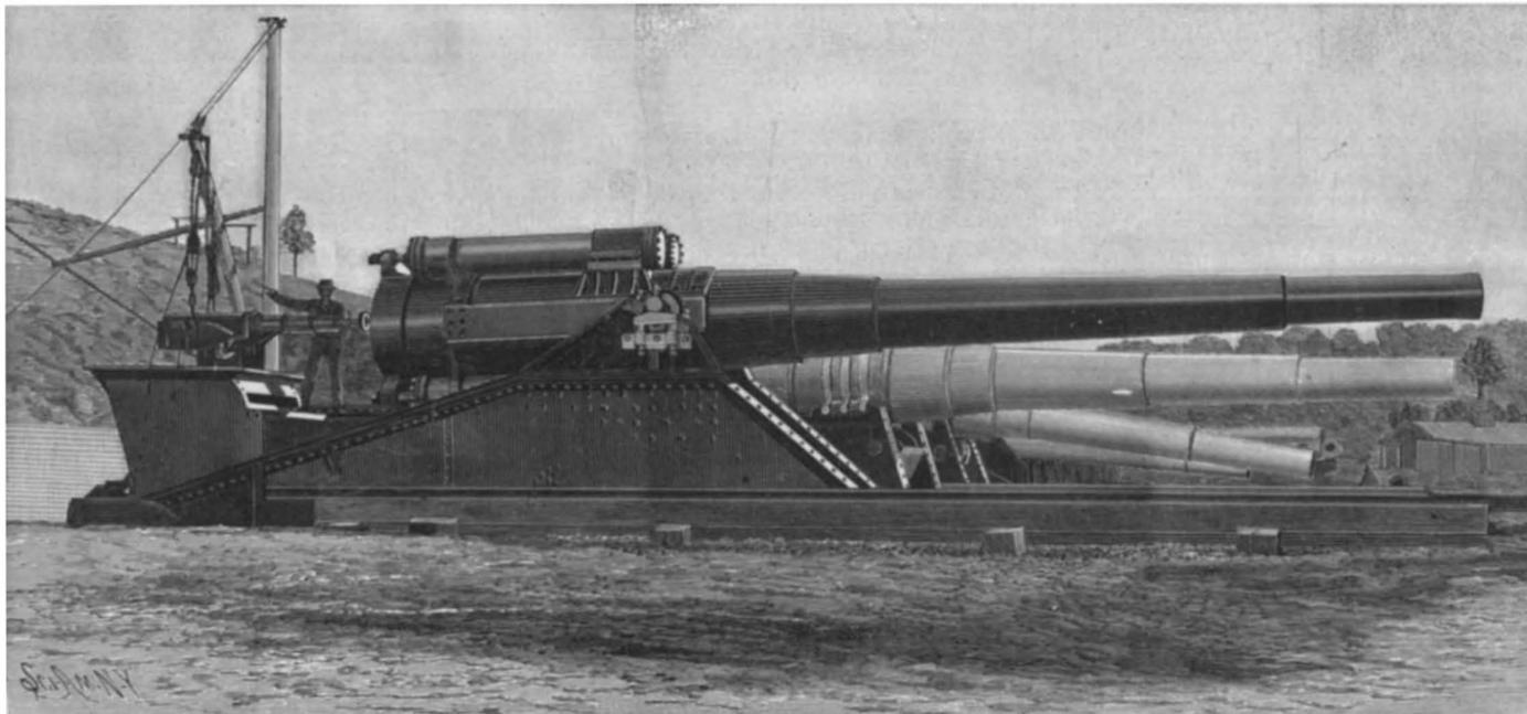
New Navy 12-inch Gun at Indian Head—Muzzle velocity, 2,854 foot-seconds; muzzle energy, 47,994 foot-tons; energy per ton of gun, 893; powder pressure, 16.5 tons per square inch.
