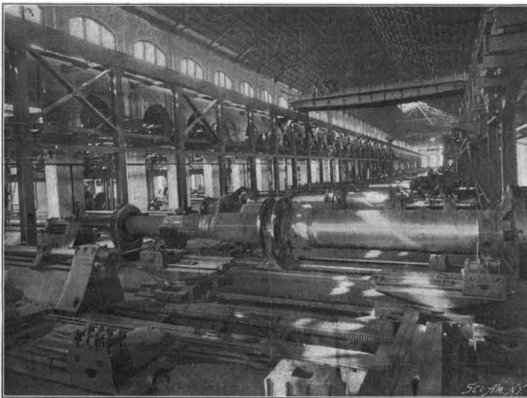
THE 16-INCH GUN IN THE LATHE BEING TURNED TO RECEIVE THE HOOPS OVER THE JACKET.
