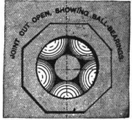
This is a picture of one of its unique ball-bearing typebars.
