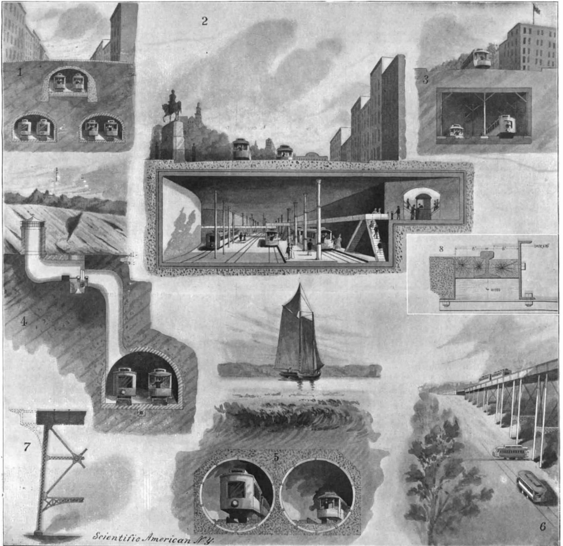
1. The four-track road in two tunnels below the Park Avenue tunnel. 2. Fourteenth Street station, looking north. 3. Two-track line below Lenox Avenue. 4. Ventilating shaft for tunnel beneath Central Park. 5. Tubular tunnels beneath Harlem River. 6. Elevated portion at One Hundred and Twenty-fifth Street. 7. Details of viaduct construction. 8. Details of track.
