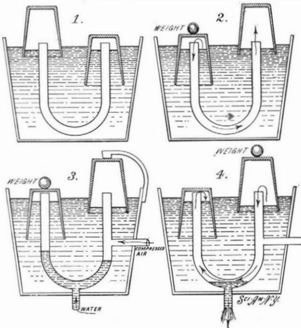
DIAGRAM ILLUSTRATING PRINCIPLES OF OPERATING THE PNEUMATIC LOCKS.
