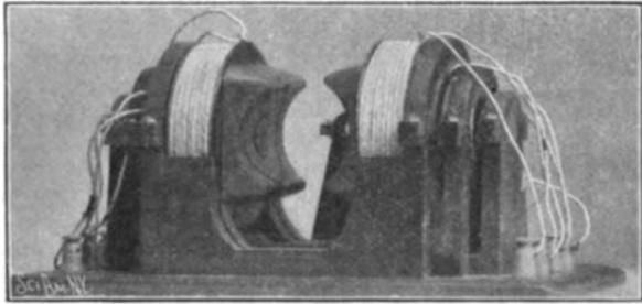
**SINGLE CIRCUIT, BIPOLAR ELECTRO-MAGNETIC MACHINE.**
