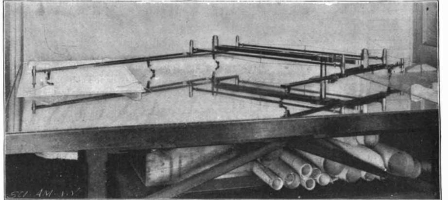
Fig. 2.—Eidograph for Reproducing Sections of Model.
