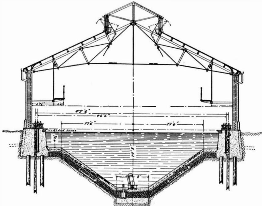
Fig. 8.—Cross-section Showing Construction of Model Basin.
