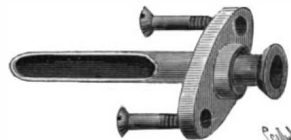
Fig. 6.—ONE OF THE IGNITING TUBES.
