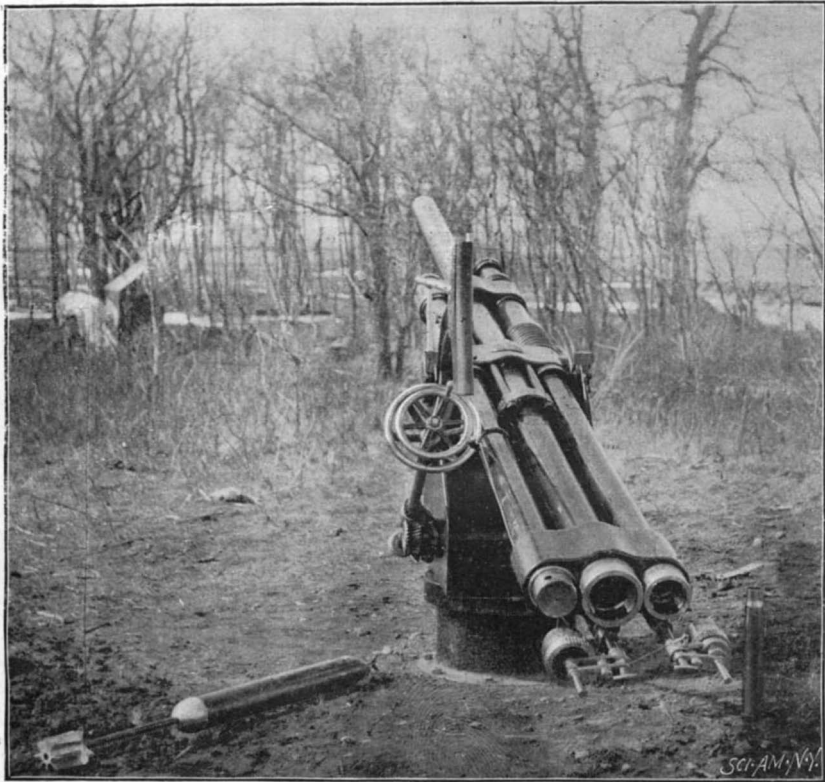
THE DUDLEY PNEUMATIC GUN—VIEW OF THE BREECH MECHANISM.
