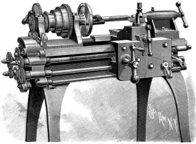
PATERSON'S SCREW-CUTTING LATHE,
