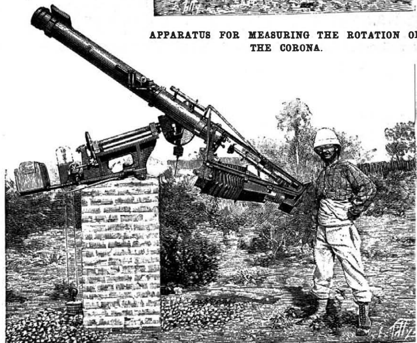
AN EQUATORIAL WITH SPECTROSCOPE ATTACHMENT.
