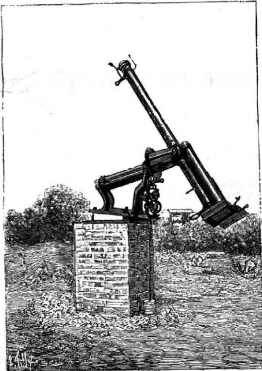
APPARATUS FOR PHOTOGRAPHING THE SOLAR CORONA.
