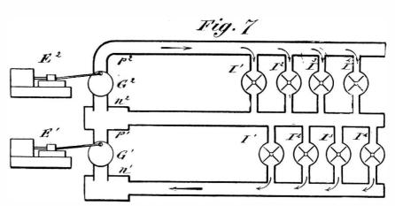
Fig. 1.—Arc Lamps in Series, Fig. 2.—Water Analogue of Series Arrangement, Fig. 3.—Incandescent Lamps in Multiple Arc, Fig. 4.—Water Analogue of Multiple Arc Arrangement, Fig. 5.—Two Multiple Arc Circuits arranged parallel. Fig. 6.—Two Multiple Arc Circuits merged into the Three-Wire System. Fig. 7.—Water Analogue of the Three-Wire System.
