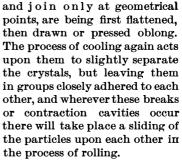
The effect of this is that the construction of the original pig metal, which appears much like compressed salt, becomes a series of fibrous-formed material, overlapping each other like brick masonry, excepting that the longitudinal sections are probably hundreds of thousands of times smaller in diameter.
