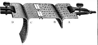
TESTING STRENGTH OF RUBBER BELTS.
