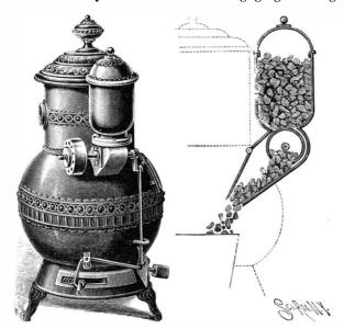
To give the grate more of a vibrating movement, a spring is arranged at one end of the slot through which the arm of the grate extends, the opposite pressures of the spring and the weight acting to increase the movement of the grate, whereby it will be effectively shaken, to keep the fire free from ashes, each time a charge of fuel is delivered into the fire pot.
