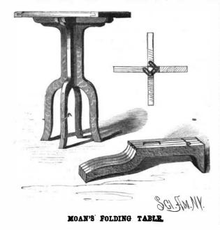
the last. When the table is arranged for use it is very strong and capable of supporting considerable weight. When it is knocked down it is very compact, and may, therefore, be readily packed for storage or shipment.
