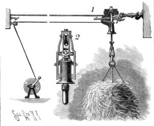
O'DELL'S HOISTING AND CONVEYING DEVICE.
