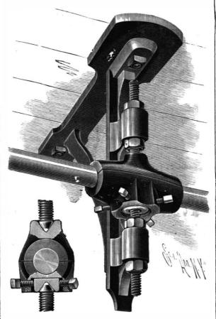
SCHNEIDER'S SHAFT BEARING OR HANGER.
