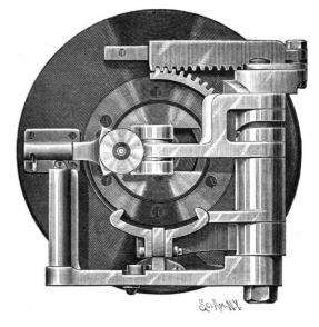
Fig. 3.-MODIFIED MECHANISM-REAR VIEW OF BREECH CLOSED.
