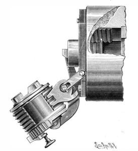
Fig. 5.-GENERAL PLAN OF BREECH, SHOWING BLOCK WITHDRAWN AND SWUNG ASIDE.
