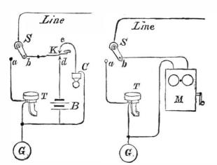
BATTERY AND MAGNETO CALLS FOR TELEPHONE LINES.
