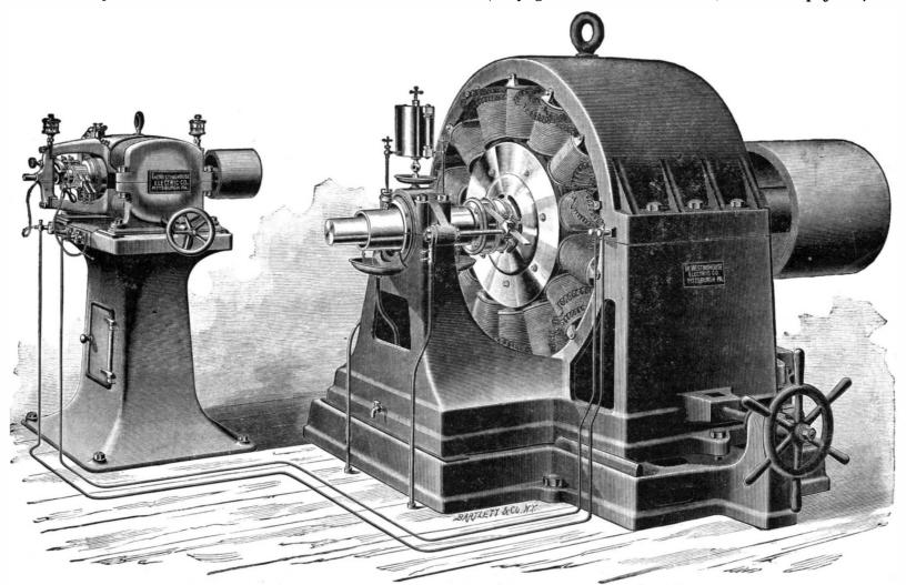
Fig. 8.-WESTINGHOUSE DYNAMO AND EXCITER-1 500 CANDLE POWER. THE ALTERNATING CURRENT SYSTEM OF ELECTRIC LIGHTING.
