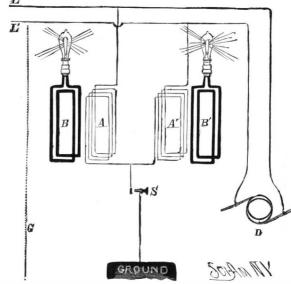
Fig. 12.-DIAGRAM OF GROUND DETECTOR.
