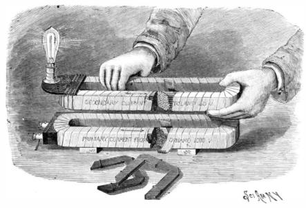
Fig. 4.-EXPERIMENT SHOWING PRINCIPLE OF CONVERTER.
