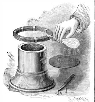
Fig. 7.—EXPERIMENT WITH A WATCH DEMAGNETIZER.
