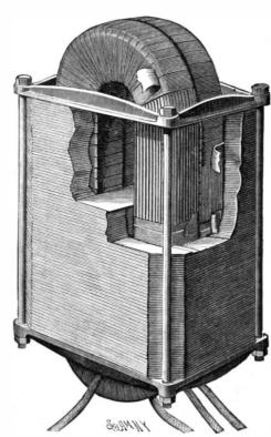
Fig. 2.-DETAIL OF CONVERTER.
