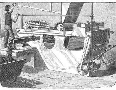
FORRESTER'S MACHINE FOR WASHING AND SEPARATING COAL.
