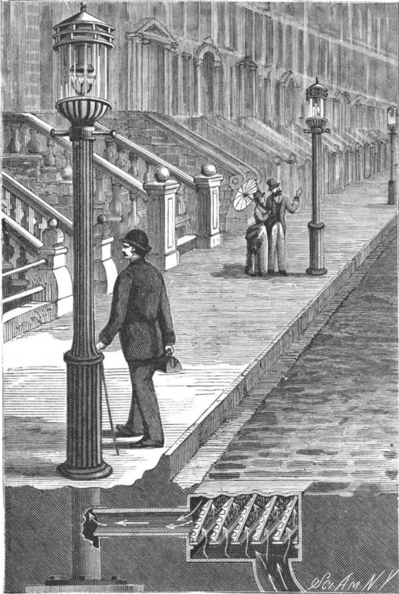
WORTHINGTON'S SEWER VENTILATOR.
