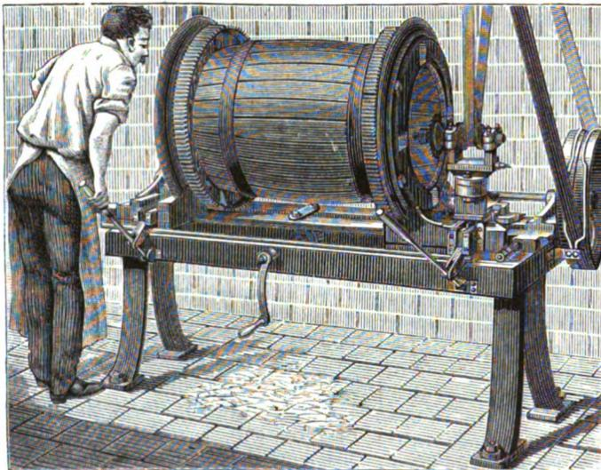
Fig. 3.—CROZING AND CHAMFERING MACHINE.
