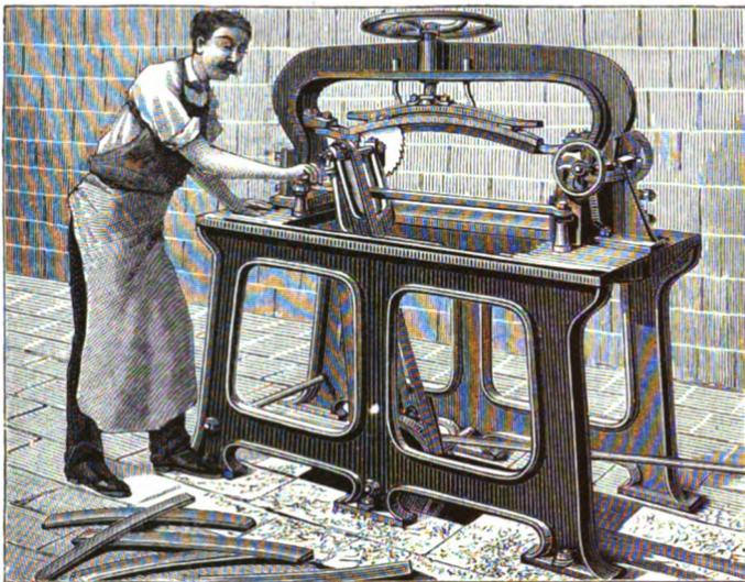
Fig. 1.—MACHINE FOR CURVING AND JOINTING STAVES.
