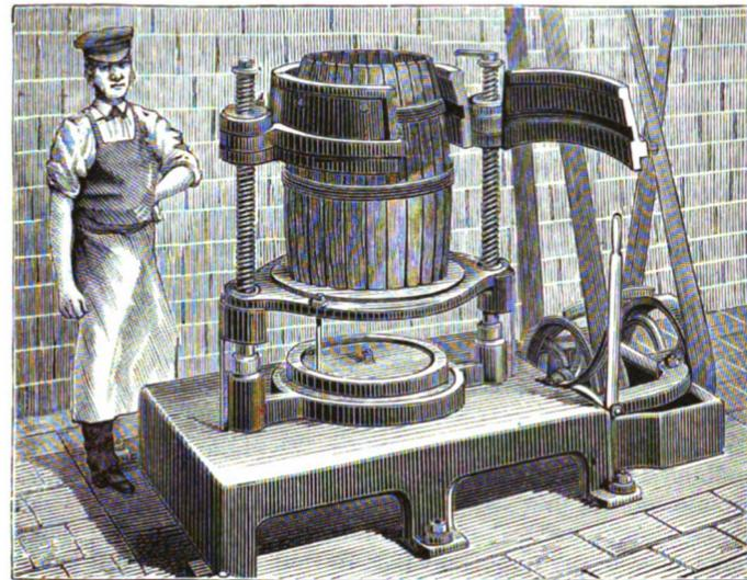
Fig. 2.—MACHINE FOR ASSEMBLING STAVES.
