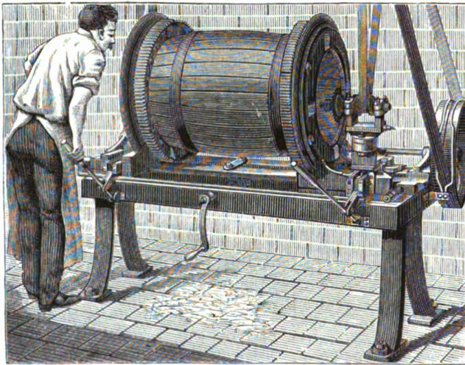
Fig. 3.—CROZING AND CHAMFERING MACHINE.
