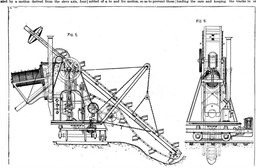
EXCAVATOR WITH ROTARY SCREEN. (Scale 1-60)
