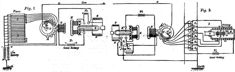
DIAGRAMS OF THE CASSAGNES SYSTEM OF TELEGRAPH TRANSMISSION.
